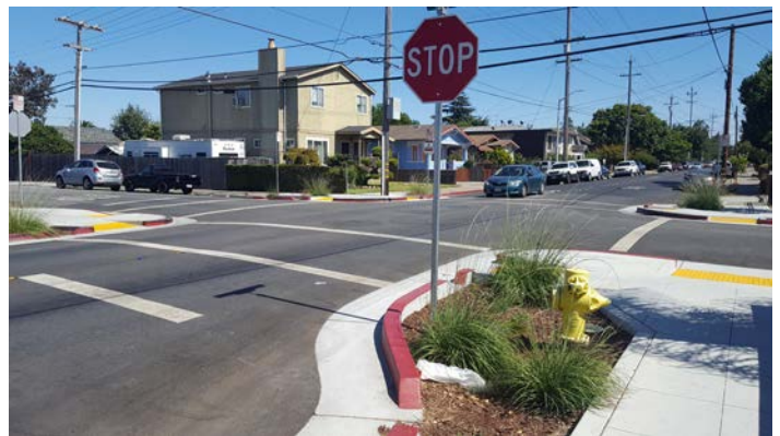
PHOTO SHOWING INTERSECTION WITH BIOSWALE BULB-OUTS
