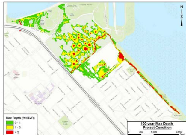
FINAL FLOOD DEPTH WITH IMPROVEMENTS
