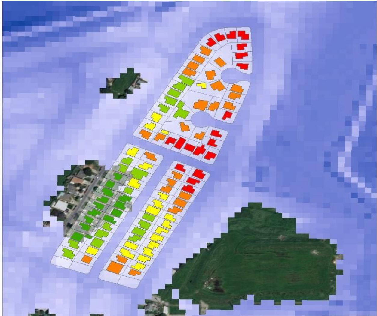
Figure 6. Illustrative example of a SURF hazard model output: for each flood scenario, the model gives average inundation depth for each building in the floodplains. Buildings that are red have a higher inundation and buildings that are dark green have no inundation.
