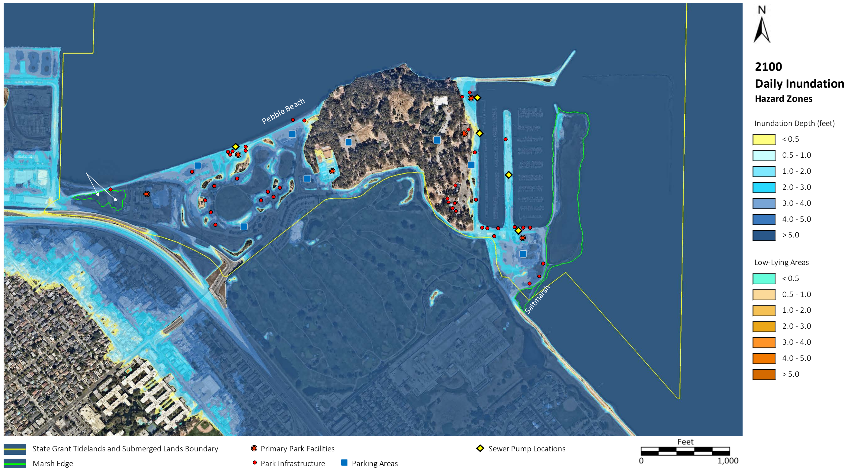
Plate 8: Flood Hazard Zones associated with Daily Inundation due to Rising Tides and 6.9 feet of SLR by 2100
