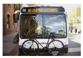
Figure 14: SamTrans Buses Accommodate Bicycles on Front Racks
