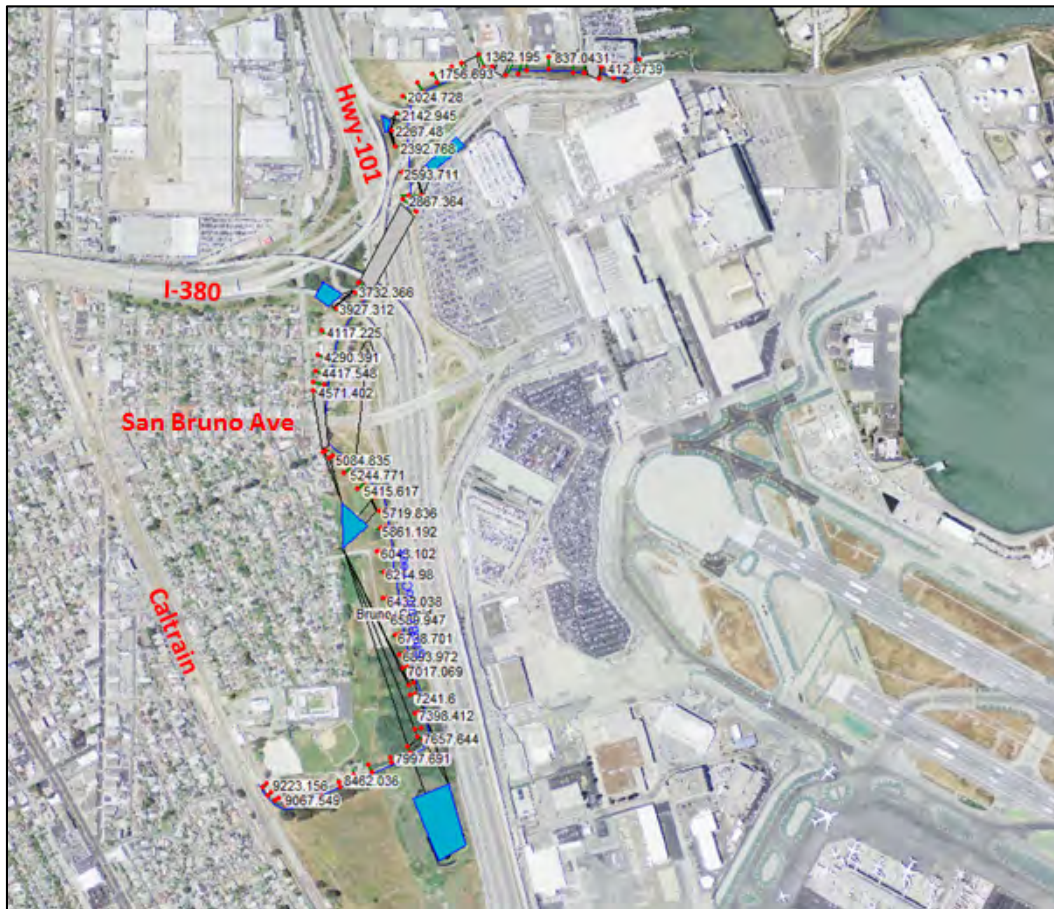
Figure 4-4. Schematic of San Bruno Creek HEC-RAS Model
