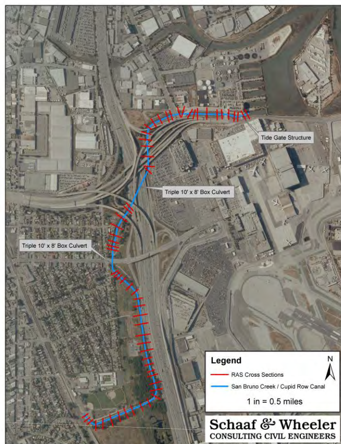
Figure 8: HEC-RAS Cross Section Locations for San Bruno Channel and Cupid Row Canal
