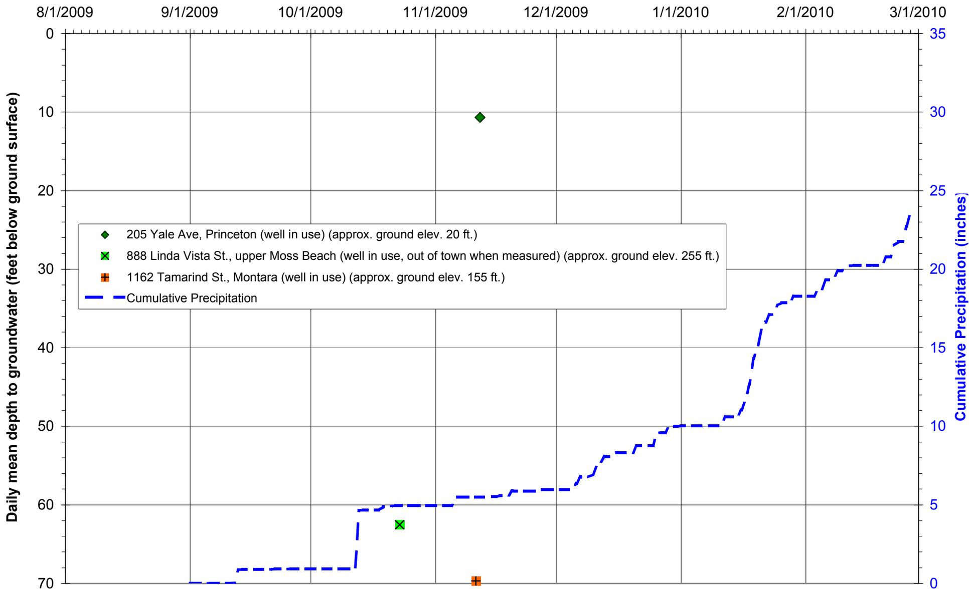
**Figure 23. Depth to water in domestic wells in used by resident, Midcoast Groundwater Study**
