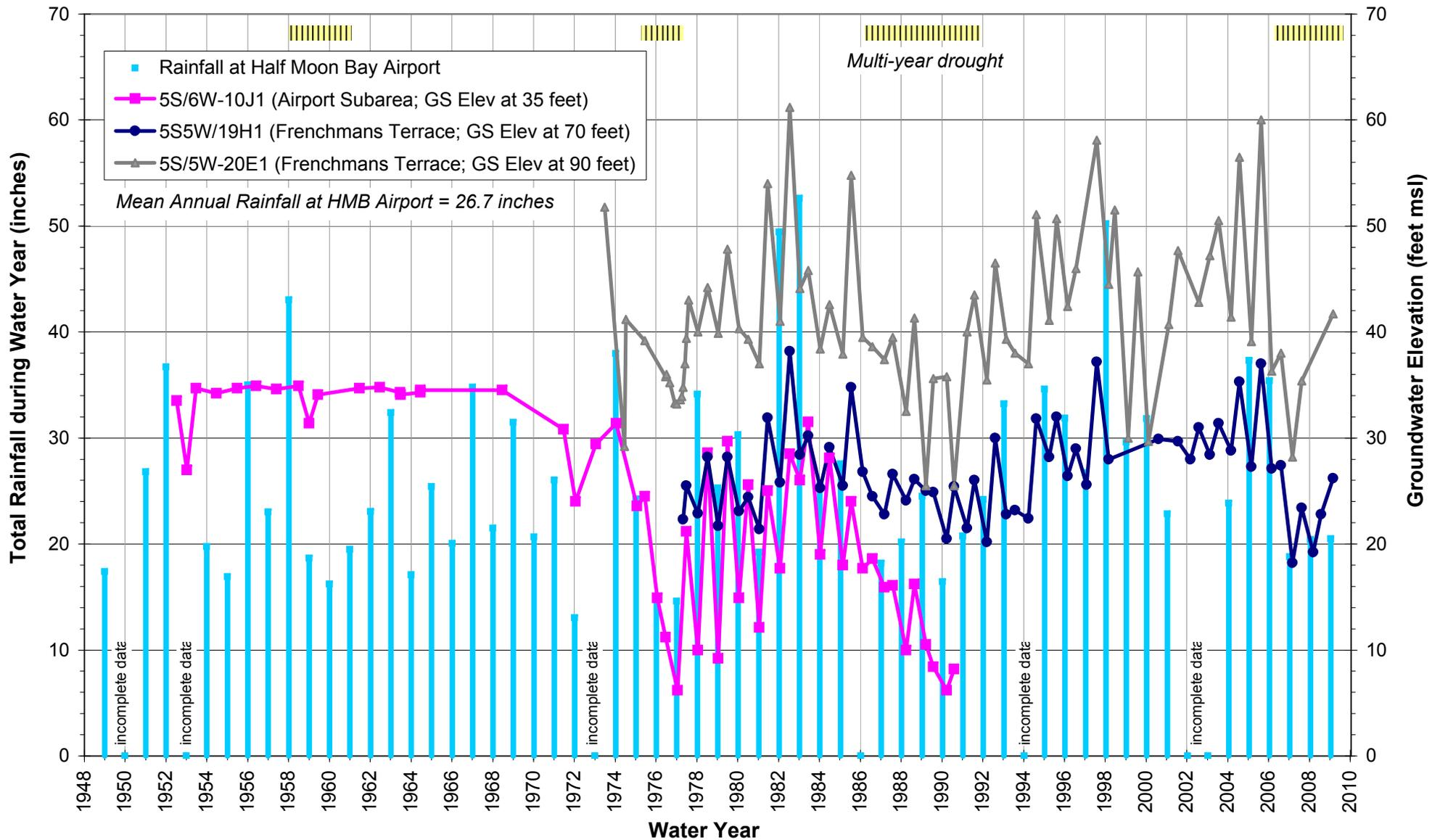
**Figure E2. Long-term record of groundwater elevations in the Airport Subarea and Frenchmans Terrace, Midcoast Groundwater Study Phase III, San Mateo County, California.** Source: Groundwater level data downloaded from DWR Water Data Library ([www.water.ca.gov/waterdatalibrary](http://www.water.ca.gov/waterdatalibrary)). 5S/6W-10J1 abandoned in 1991. Rainfall data from Half Moon Bay Airport (NOAA NCDC Station 43714), annual totals not shown for years with missing data.
